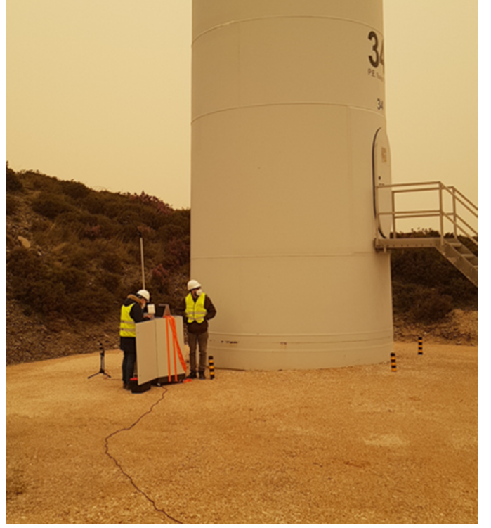
Fig. 3. Acoustic Monitoring System under a Wind Turbine
