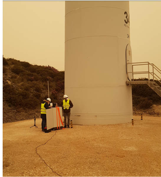
Fig. 3. Acoustic Monitoring System under a Wind Turbine
