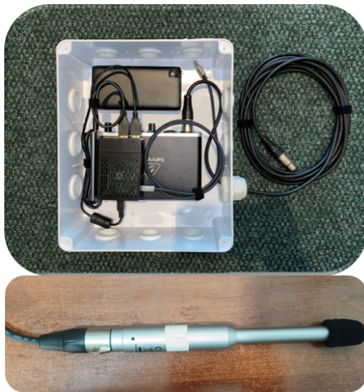
Fig. 2. Generic Acoustic Monitoring System
